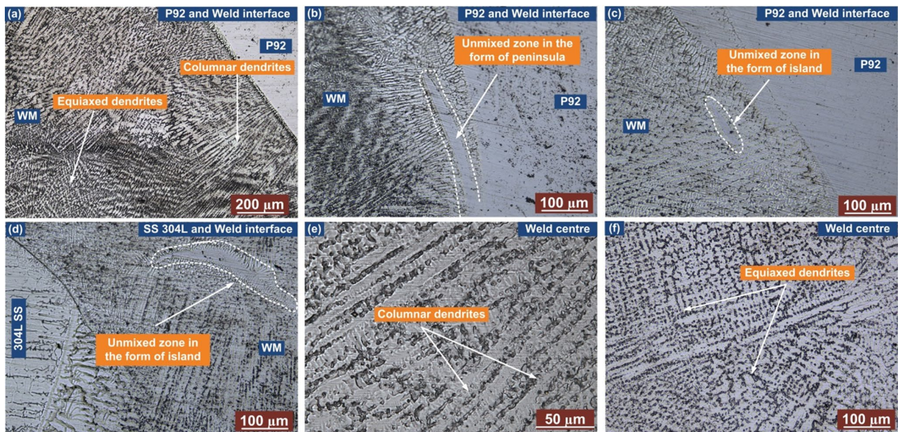
Fig. 16 In as-weld state optical microstructure of the ERNiFeCr-2 weld metal a–c P92 and weld interface, d 304L SS and weld interface and e, f weld centre for narrow groove design
