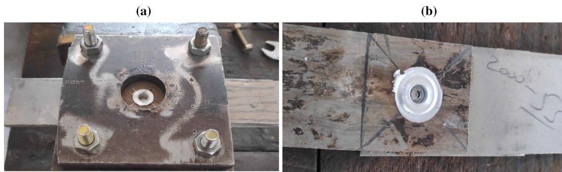
Fig. 3 FSSW of AA7075-T651 with Ti-6Al-4V alloy, a assembly mechanism b welded sample according to JIS Z3136 standard
