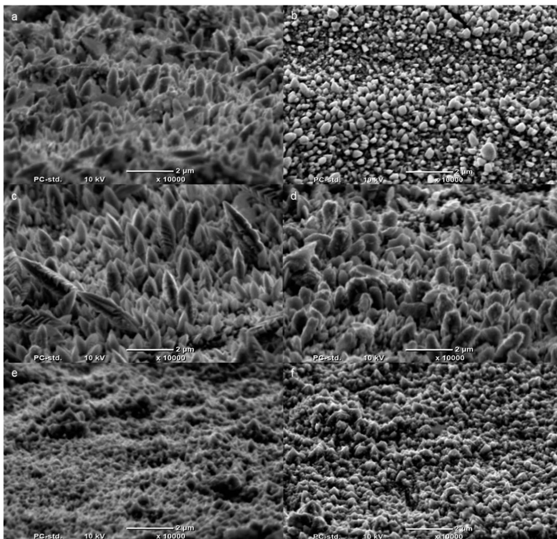
Fig. 9 Coating obtained at 500 mT in (a, c, e) perpendicular and (b, d, f) parallel magnetic field (magnification: \times 10k ) from the electrolyte: A (a, b), B (c, d), and C (e, f)
