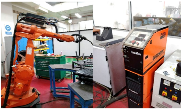
Fig. 1 ABB IRB 2400/16 Robotic welding Machine (left) and KEMMPI ProMig 540 MXE (right)
