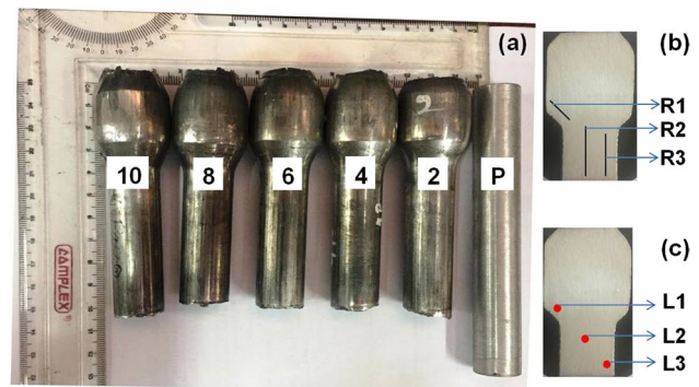
Fig. 2 a Parent AA 6063 [annealed (P)] and CEE-processed specimens (2–10 passes), b R1, R2, and R3 regions identified for hardness measurements, and c L1, L2, and L3 regions in the CEE-processed specimens considered for microstructure examination
