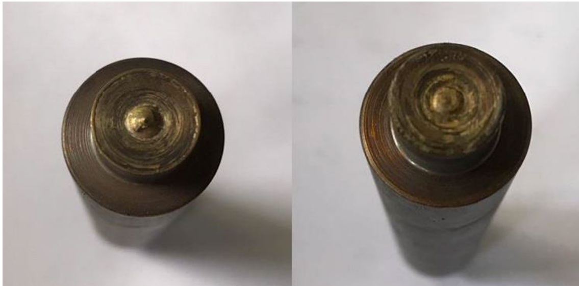
Fig. 7 Tools after FSP at rotational speed of 1120 rpm
