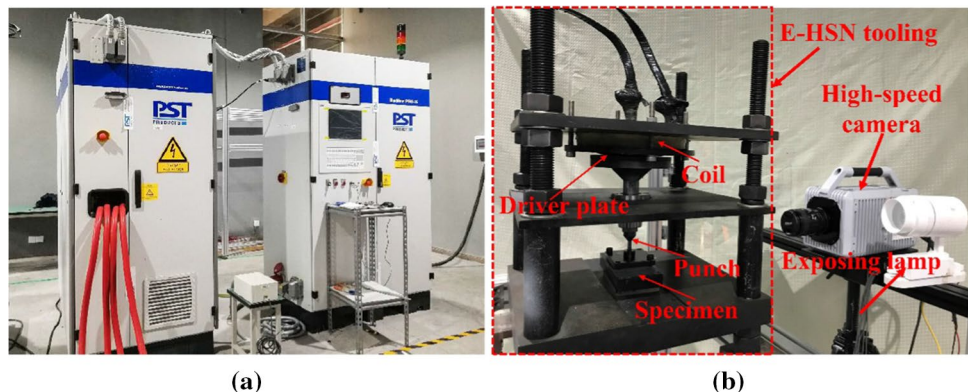
Fig. 4 The diagram of the PST magnetic pulse generator, E-HSN tooling and high-speed camera: a PST magnetic pulse generator, b the E-HSN tooling and high-speed camera
