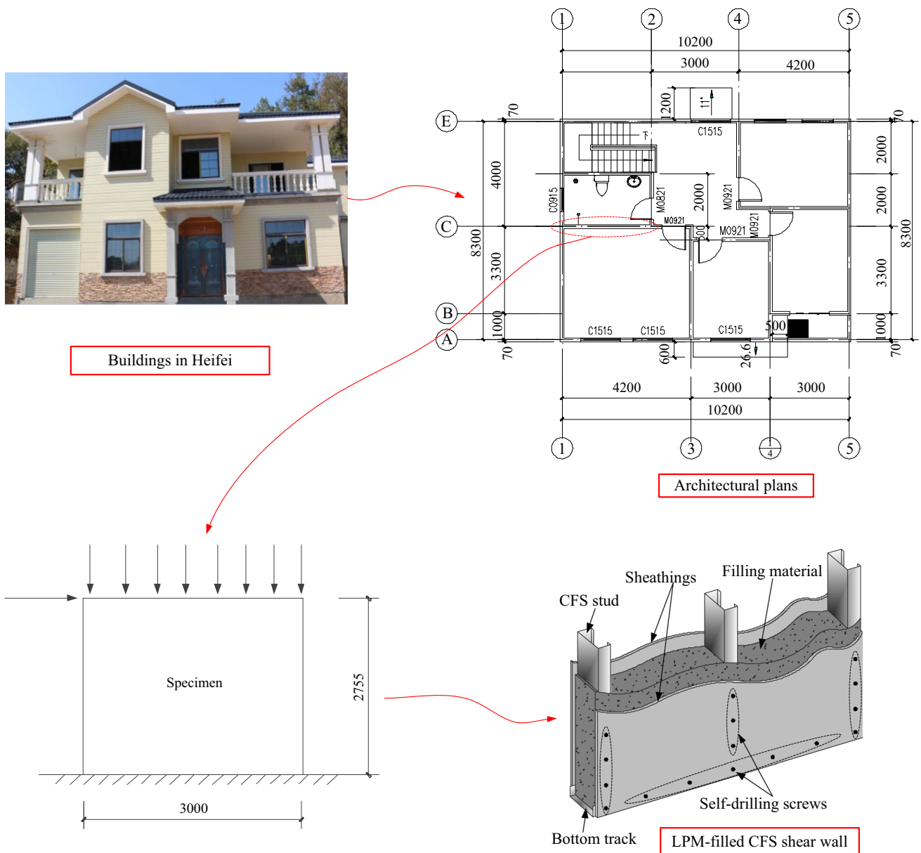
Fig. 1 Application of LPM-filled CFS wall in building
