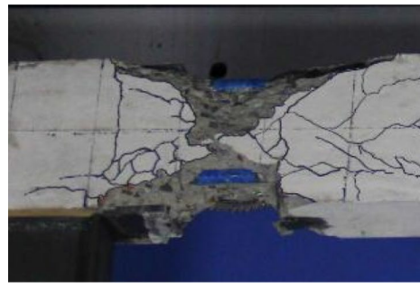
(c) Plastic hinge of the beam at the left column
