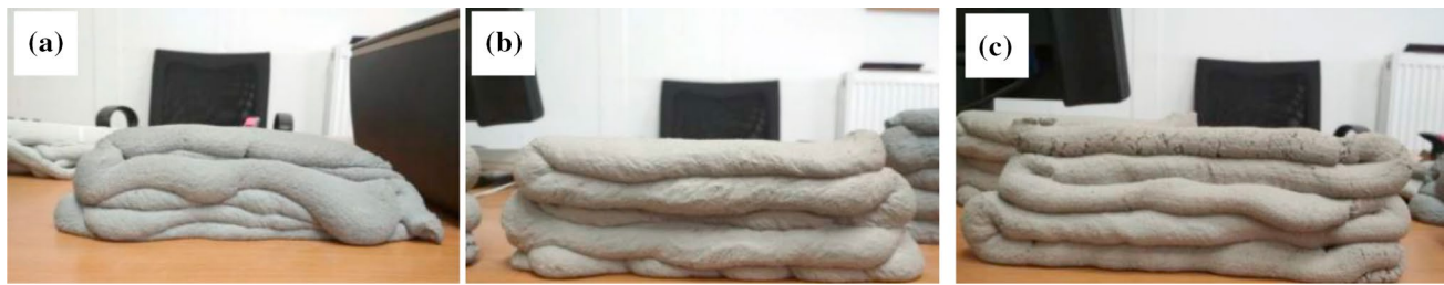
Fig. 8 Limestone and cement mixture with a high, b moderate, and c high workability level. As seen from the figure, this mixture is not considered printable [58]
