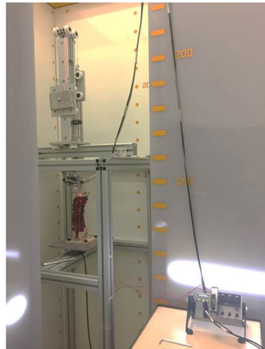
Fig. 2 Specimen mounted on the specially designed testing apparatus equipped with an EOS imaging system for motion tracking
