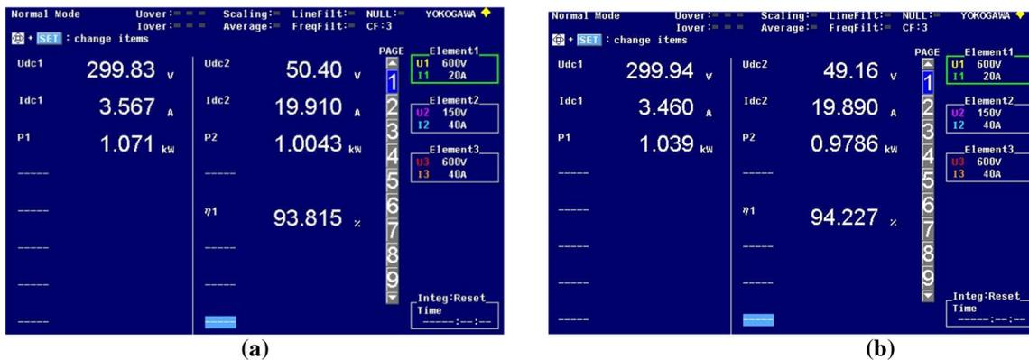
Fig. 16 Measured Efficiency at input voltage 300 V, output voltage 50 V, and output power 1.0 kW: **a** conventional converter; **b** proposed converter
