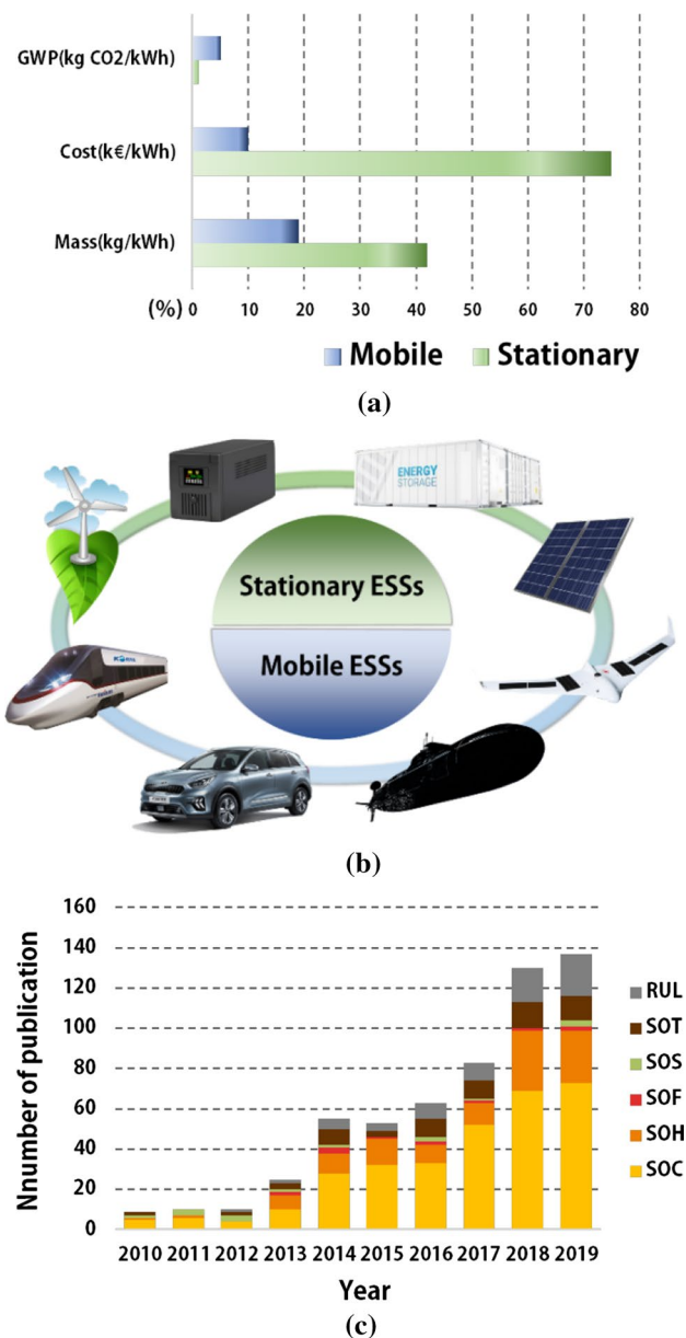
Fig. 1 Overview of ESSs and battery states: a energy supplied for different examined systems (normalized per kWh) [5], b classification of stationary ESSs and mobile ESSs; c number of publications focused on battery states in the last 10 years
