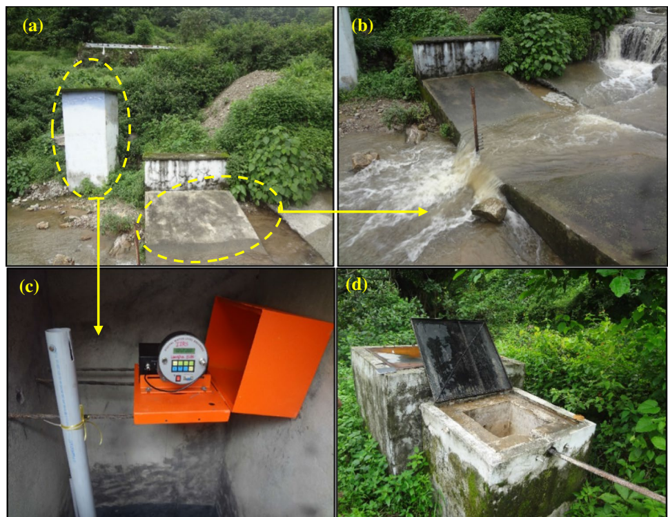
Fig. 4 Instrumented gauging site at the watershed outlet: stilling well (a), weir structure (b), digital water level recorder (c), and sediment sampling tank (d)
