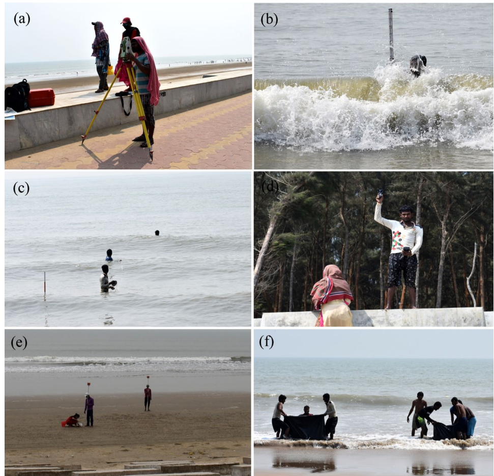
Fig. 2 Data collection (a) through Total station survey; measurements of (b) breaking wave height, (c) wavelength and frequency, and (d) wind speed; and collection of (e) sediment sample from the beach (f) and sediment volume from successive swash and backwash in different aspects of beach morphology, hydrodynamics and sedimentology
