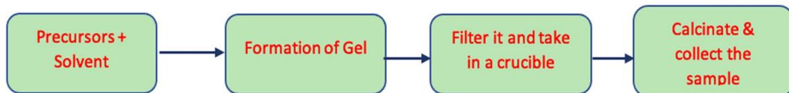
Fig. 3 Flow chart for sol–gel method
