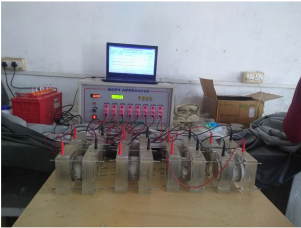
Fig. 2 RCPT test setup
