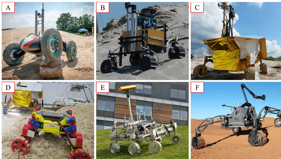
Fig. 1 Modified wheeled travel. A SCARAB; B El-Dorado-II-B; C RP15, the precursor to VIPER; D Mini-RP15, E Rosalind Franklin Rover; F SherpaTT. A Adapted with permission. Copyright 2019, NASA. B Adapted with permission [16]. Copyright 2013, Wiley Periodicals, Inc. C Adapted with permission [32]. Copyright 2015,
