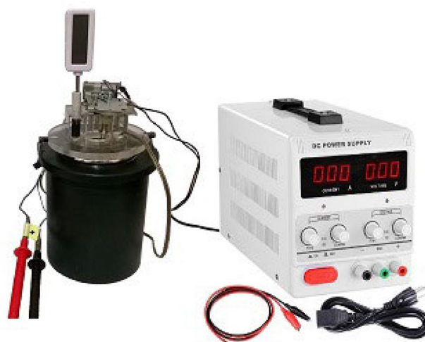
Fig. 1 The experimental device used for heat capacity measurement
