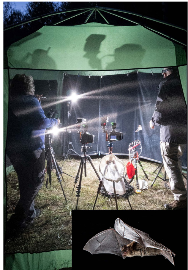
Fig. 8 SLF and MBF in a screen tent set up as a studio for photographing flying bats. The tent is 2 m by 4 m by 2.5 m tall. A little brown myotis ( Myotis lucifugus ) can be seen flying just above the four beams. Two of 8 flashes are obvious, as are three cameras each on a tripod. There is a hand net leaning against one tripod for recapturing the bat. A black cloth has been hung from one side of the tent for a background. We had pitched the tent near an abandoned mine used by swarming bats. Tent photo by Lily Hou. Inset photo shows one of the photographs of the little brown myotis taken with this setup by S. L. Fenton and M. B. Fenton
