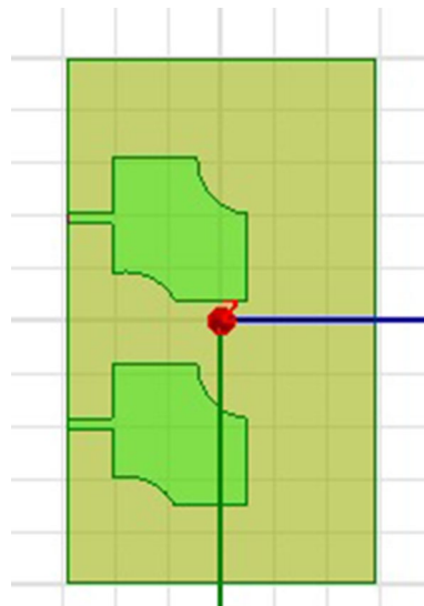
Fig. 4 Designed 2 × 1 MIMO antenna with partial circular cuts
