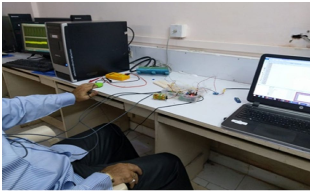
Fig. 4 Acquisition of ECG and PPG from subject using hardware prototype model
