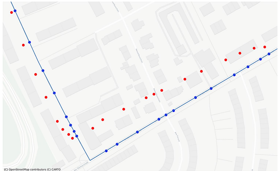
Fig. 1 GPS recorded points (red) and matched points (blue). The blue line shows the corresponding trajectory found by map-matching. basemap: ©OpenStreetMap ©CARTO
