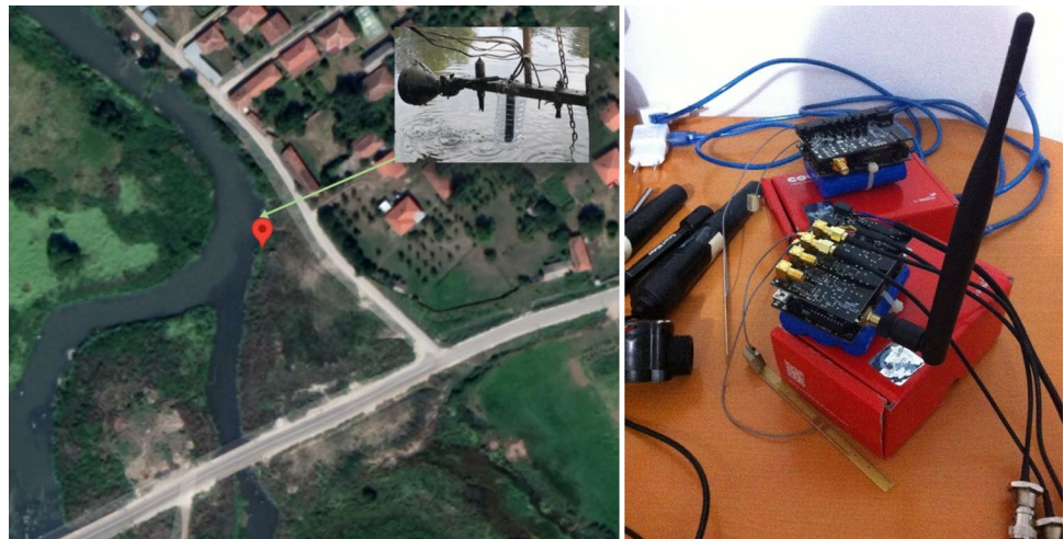
Fig. 4 System architecture: implementation of proposed data stream management model in WQMS
