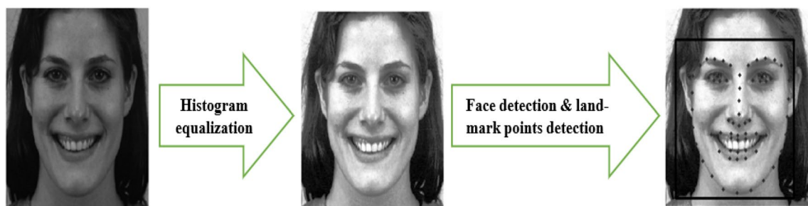
Fig. 4 Three preprocessing steps: histogram equalization, face detection and landmark points detection
