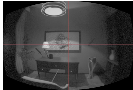
Fig. 2 Luminance channel of an image captured by I29 from HTC Vive Pro Eye, using ProMetric.
