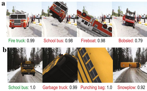
Fig. 1 Examples of geometric transformations that make seemingly easy recognition tasks challenging for computer vision algorithms. The above is a demonstration by Alcorn et al. [1] of prediction performance of Inception—V3 under different viewing conditions of a a fire truck and b school bus. Images courtesy Ref. [1], © IEEE 2019
