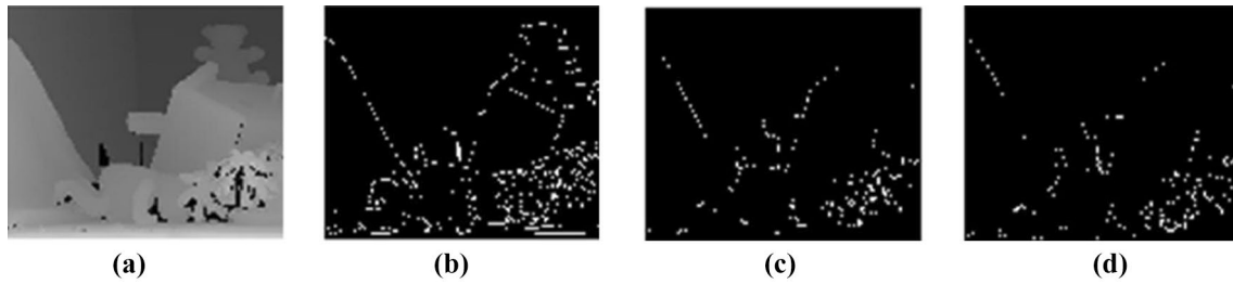
Fig. 5 a Original image and its corresponding processed image, b Canny operator, c Prewitt operator, and d Roberts operator
