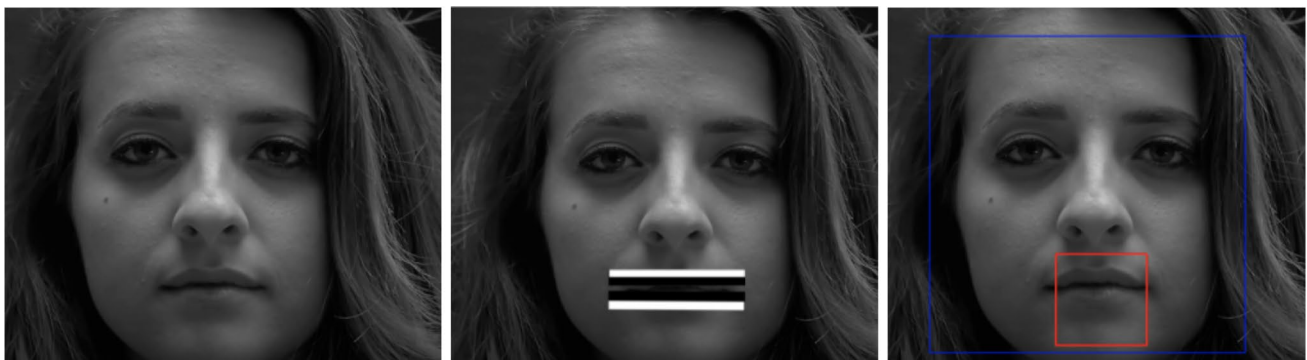
Fig. 2 Progress from initial Haar-Feature detection from calculated intensity differences to completed lip closure detection
