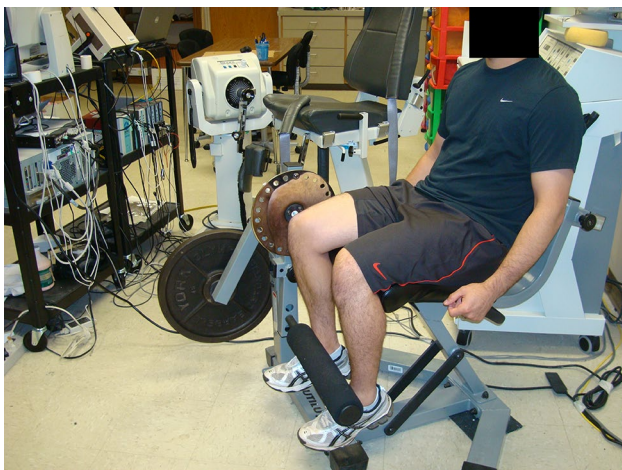
Fig. 3 Dynamic constant external resistance assessment set-up with isokinetic dynamometer on the background
