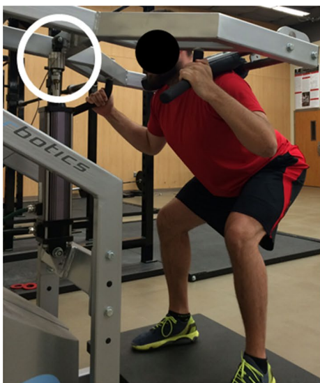
Fig. 1 Examples of the isometric squat data collection and analysis procedures. The image on the left shows a younger adult male performing an isometric squat as described herein. The load cell used to acquire the torque data has been circled. On the right, an exam-
