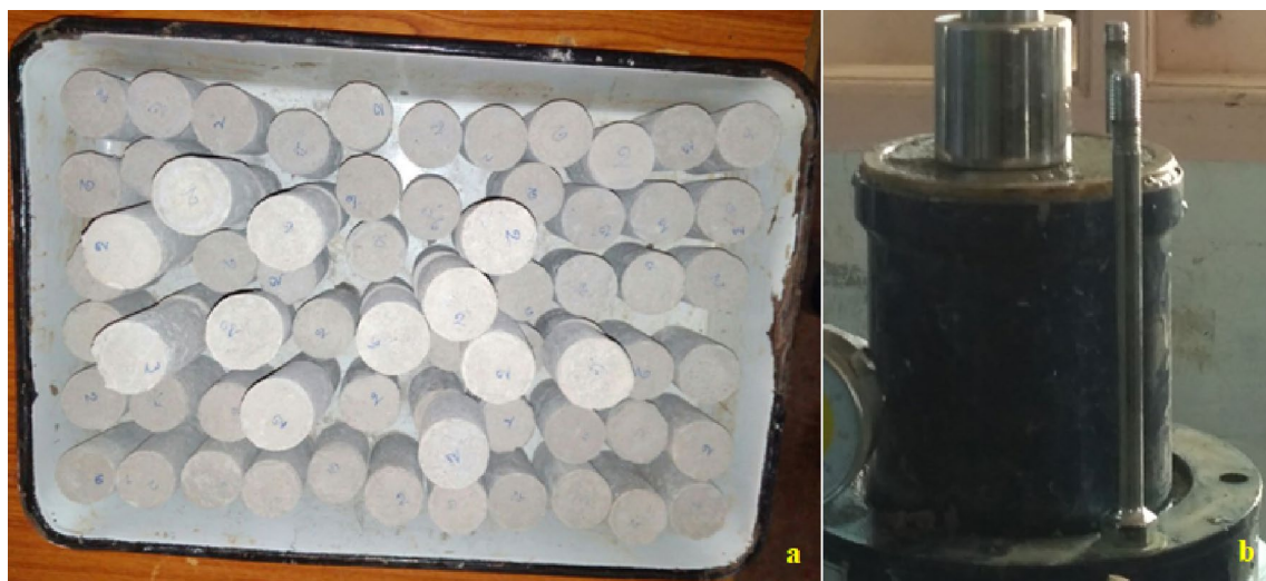
Fig. 4 Sample prepared for strength testing. a Sample for UCS test, b sample prepared for CBR test
