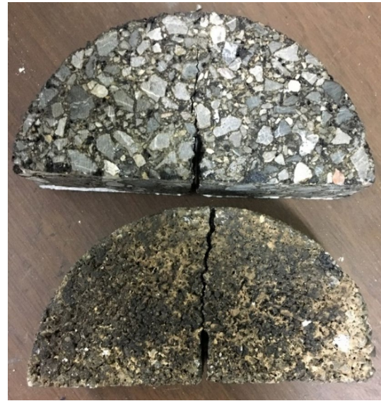
Fig. 5 SCB Sample made in this study
