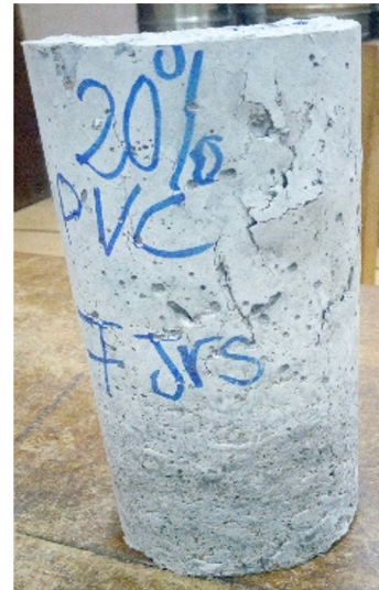
Fig. 7 Cylindrical specimen after compression test
