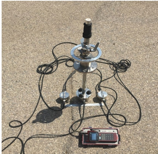
Fig. 3 The positions of geophones and the loading plate in this study
