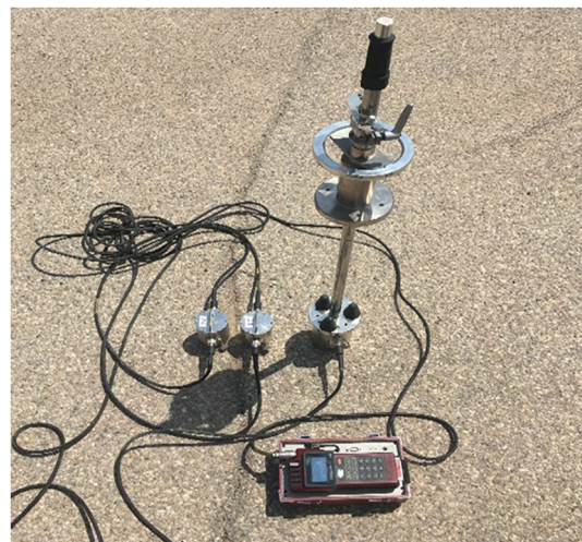
Fig. 1 The position of geophones and the PFWD device for data collection
