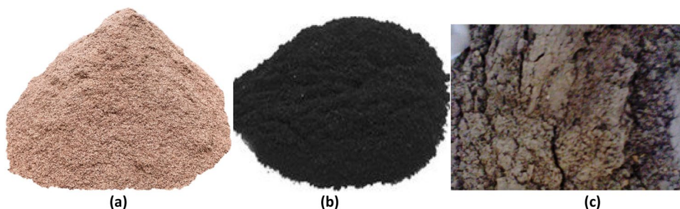
Fig. 1 Materials for the experiment. a Saw dust waste; b saw dust ash; c soil–saw dust ash mixture
