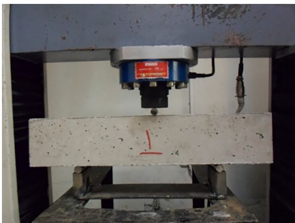
Fig. 9 Three-point bending test by universal testing machines
