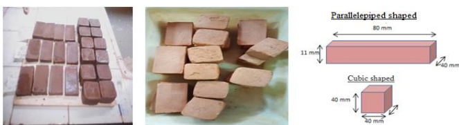
Fig. 4. Parallelepiped and cubic samples before and after firing and sketch of the samples respectively according to the standard NF EN 771-1.
