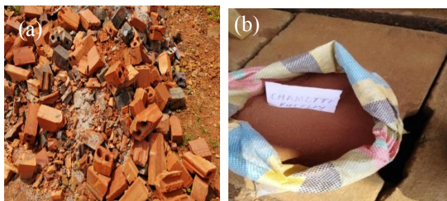
Fig. 2. (a) broken burnt bricks and (b) burnt brick powder.
