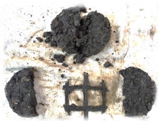
Fig. 12. Geogrid not adhered to the cold asphalt mixture (CMA).
