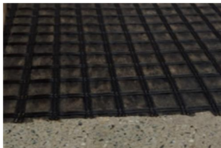
Fig. 1. Geogrid used in the research.
