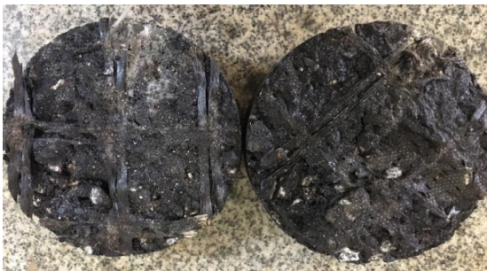
Fig. 11. Geogrid adhered to the hot asphalt mixture (HMA).
