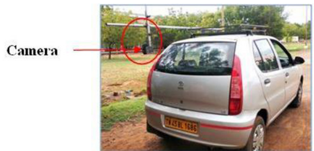
Fig. 5. Data collection setup for vision-based approach.
