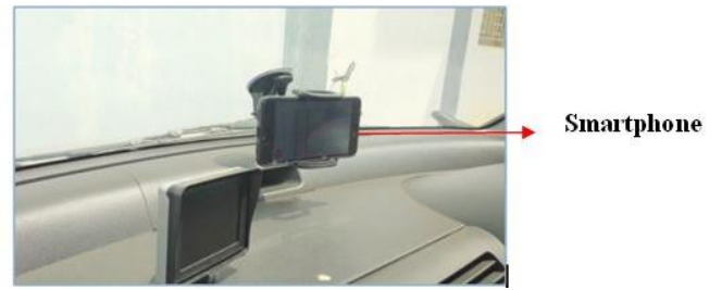
Fig. 4. Data collection setup for vibration-based approach.
