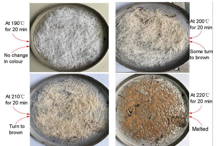
Fig. 6. The change of surface of waste nylon filament.
