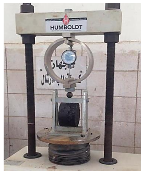
Fig. 7. Indirect tensile strength test.
