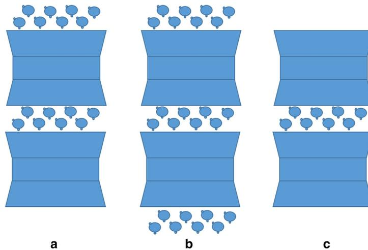
**Fig. 5** Various possible configurations of interlayer H<sub>2</sub>O molecules in a two-layer smectite crystallite
