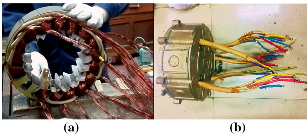
Fig. 13 The stator winding of multi three-phase unit machine a Winding process b Stator winding connections
