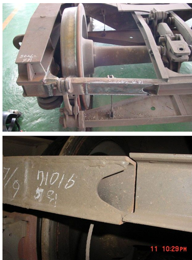
Fig. 3 Bogie frame of the freight train and its fracture at the end beam
