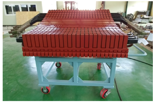
Fig. 4 Stator core with inserted bars on a carrier
