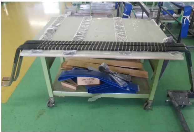
Fig. 2 Manufactured bars with sparsely wound outer corona-preventive tape (Type-C bars)
