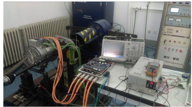
Fig. 12 Experimental bench for IPMSM system
