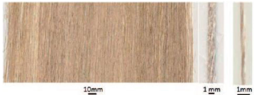
Fig. 4 Three different flax fiber bundle types: on the left side — hackled flax (fiber aligned, width of about 25 cm, 30,000 tex); middle — flax roving (more stretched, but there is a low amount of twist, 280 tex); on the right side — flax yarn (twisted, 83.3 tex) (Baets et al., 2014)
