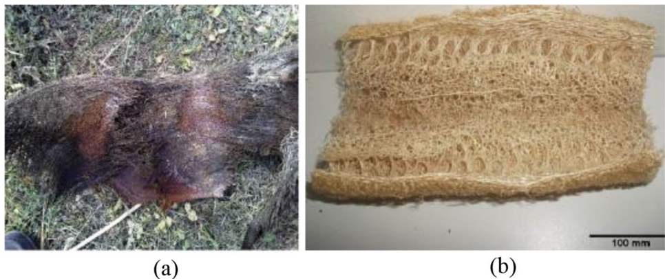
Fig. 7 Fibrous structure from nature ligaments: a date palm mesh (Benaimeche et al., 2018), b sponge gourd ( Luffa cylindrica L.) (Querido et al., 2019)
