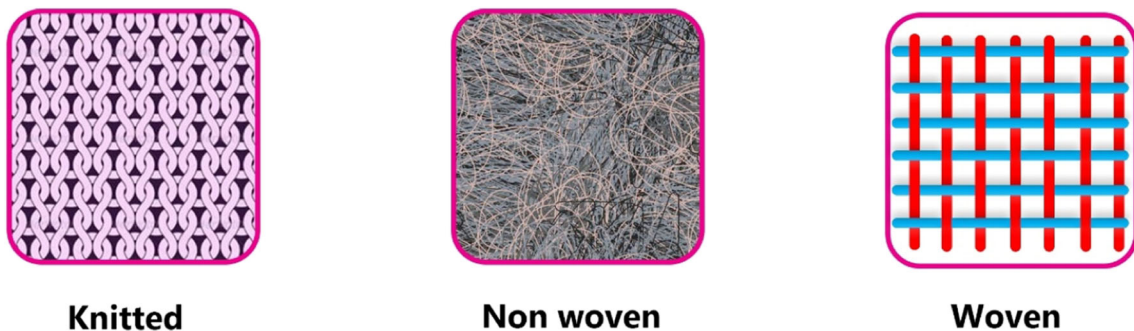
Fig. 5 The structural differences between nonwoven and woven fabrics
