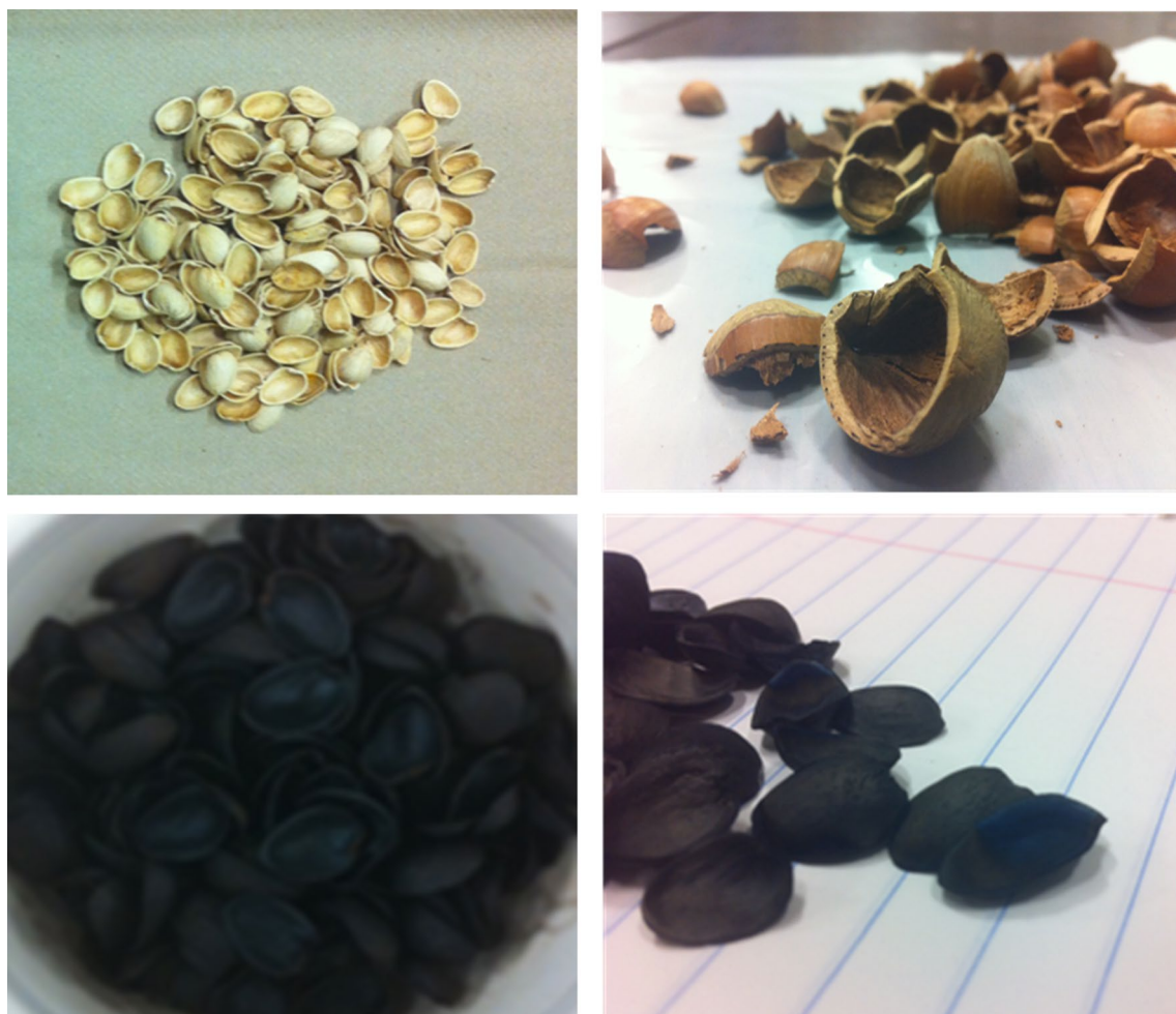
Fig. 1 Images showing a the pistachio shells, b acorn shells, c pistachio shells after carbonization and d the same pistachio shells after activation with KOH solutions prior to the grinding
